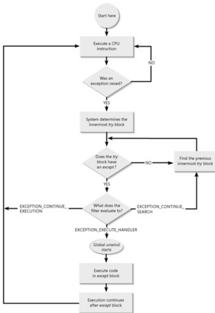
Figure 24-1: How the system processes an exception
